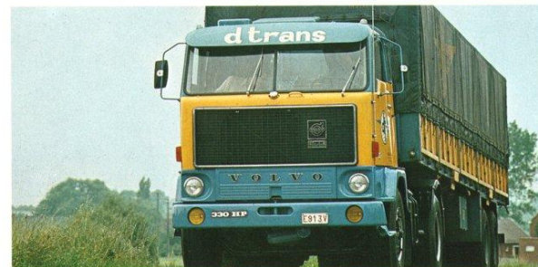
An F 89-32 4x2 with two-axle semi-trailer. TD 120 engine, SR 61 gearbox, double reduction final drive.
