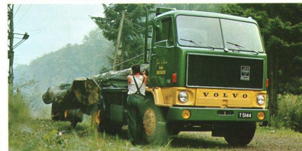
An F 89-32 4x2 with two-axle folding trailer for timber transport. TD 120 engine, SR 61 gearbox, single reduction final drive with hub reduction.
