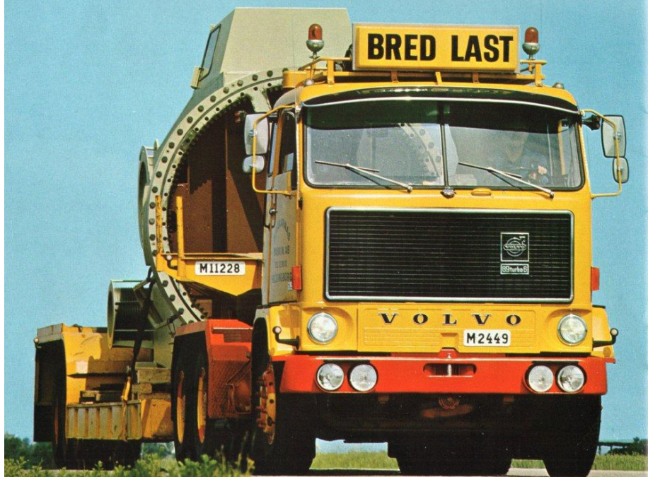
An F 89 6x2 tractor unit with a special drop-bed semi-trailer for the transport of heavy machinery
