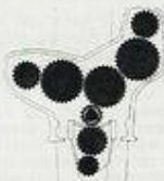
All the timing gears are manufactured of high-quality steel. The gear drive ensures more reliable running and enables a more compact design.
