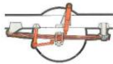
Front parabolic springs combined with double-acting telescopic shock absorbers.
